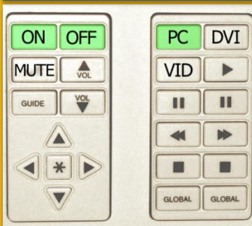
Figure D: Wall Control Panel
