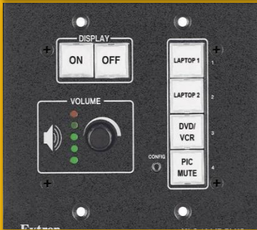
Figure A: Extron Control Panel
