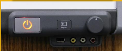
Figure B: SMART Board Control Panel
