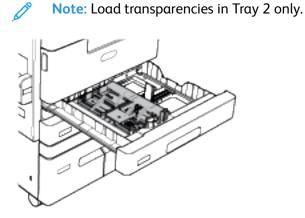
• For short-edge feed, insert letterhead and pre-printed paper face down with the top edge to the left. Load hole-punched paper with the holes toward the rear of the printer.
