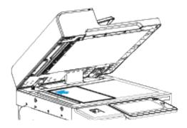
• For multiple, single, or 2-sided pages, use the duplex automatic document feeder. Remove all staples and paper clips from the pages. Insert the original documents face up in the duplex automatic document feeder, with the top of the page entering the feeder first. Adjust the paper guides so that they fit against the documents.
