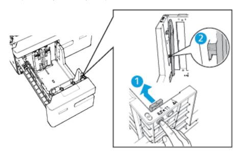
6. To adjust the rear right-side paper guide, press the pin on the outside of the tray inward. To release the black paper guide from the side of the tray, gently pull out the guide, then pull it up. Move the guide to the new position, align the bottom hook of the guide with the new position, then press the guide firmly into place.
