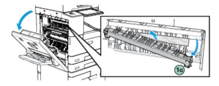
3. In the left side door, use the green tab to lift cover 1b, then carefully remove any jammed paper.
