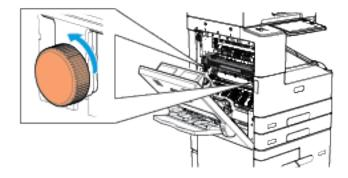
5. Pull out the used fuser module.
