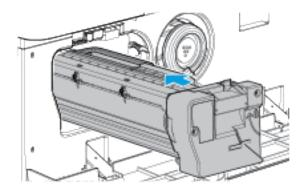
10. To latch the new print cartridge into place, rotate the orange lever clockwise.
