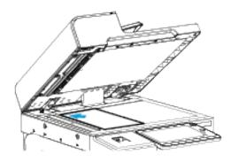
• For multiple, single, or 2-sided pages, use the duplex automatic document feeder. Remove any staples and paper clips from the pages. Insert the original documents face up in the duplex automatic document feeder, with the top of the page entering the feeder first. Adjust the paper guides so that they fit against the original documents.
