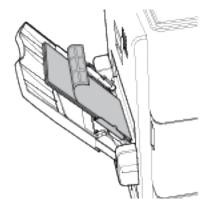
**Note:** Do not load paper above the maximum fill line. Overfilling the tray can cause the printer to jam.
