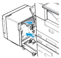
2. Open the left side door of the printer. Remove any jammed paper from the left side door areas.
