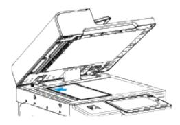
• For multiple, single, or 2-sided pages, use the duplex automatic document feeder. Remove any staples or paper clips from the pages. Insert the original documents face up in the duplex automatic document feeder, with the top of the page entering the feeder first. Adjust the paper guides so that they fit against the document originals.
