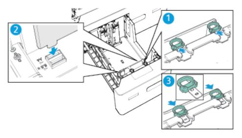
4. To adjust the rear paper guide, slide back the green clips, then lift the rear paper guide gently to release it from the tray. Move the guide to the new paper-size position. Align the tabs at the top and bottom of the guide with the corresponding slots on the tray, then slide forward the green clips.
