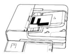
Note: To insert special pages into the job, in Tray 7, load the pages face up and rotated 180 degrees from the pages in the automatic document feeder.
