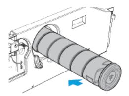
6. To lock the toner cartridge into place, rotate the orange toner cartridge locking lever clockwise.
