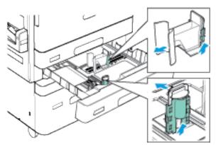
• For C5 envelopes with the flap on a short edge, load the envelopes face up with the flaps closed, and the flaps toward the front of the printer.
