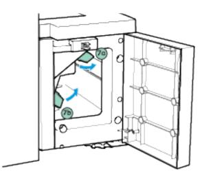
Ensure that you have removed all jammed paper, and that jam area covers are closed correctly.
