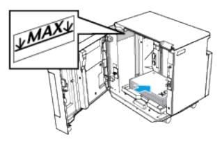
Note: Do not load paper above the maxiumum fill line. Overfilling can cause paper jams.
