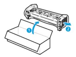
5. Lift the orange cartridge handle slightly and pull the cartridge half out of the printer.
