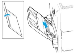
• For envelopes with the flap on a short edge, load the envelopes face down with the flaps closed, and the flaps toward the front of the printer.
