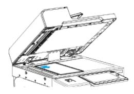
• For multiple, single, or 2-sided pages, use the duplex automatic document feeder. Remove all staples and paper clips from the pages. Insert the original documents face up in the duplex automatic document feeder, with the top of the page entering the feeder first. Adjust the paper guides so that they fit against the documents.
