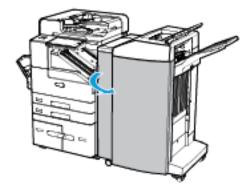
2. Slide the hole-punch waste container out of the finisher.
