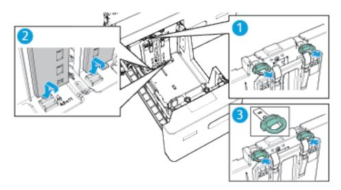
5. To adjust the front right-side paper guide, press the pin on the outside of the tray inward. To release the black paper guide from the side of the tray, gently pull out the guide, then pull it up. Move the guide to the new position, align the bottom hook of the guide with the new position, then press the guide firmly into place.
