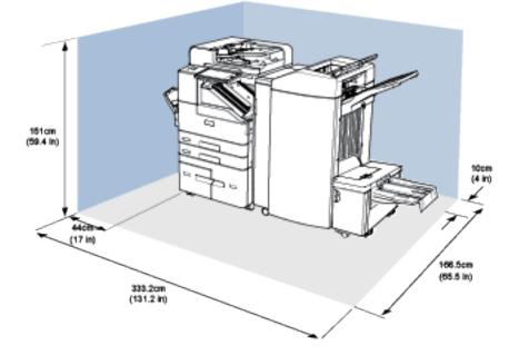
Clearance Requirements for Configuration with High Volume Finisher, Booklet Maker, CZ Folder and High Capacity Feeder
