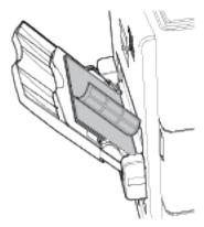
• For short-edge feed, load labels face down with the top edge leading into the printer:
