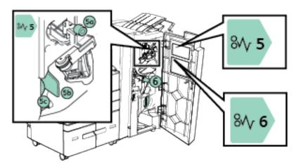
Ensure that you have removed all jammed paper, and that jam area covers are closed correctly.
