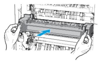
8. To fasten the fuser module, rotate the orange thumbscrews clockwise.
