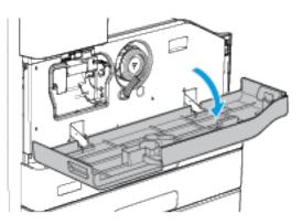
2. To release the toner cartridge, rotate the orange toner cartridge locking lever counterclockwise.
