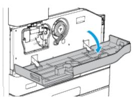
2. Rotate the orange print cartridge locking lever counterclockwise until it clicks. The lever is to the right of the print cartridge unit.
